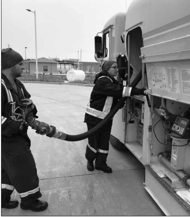
Private Dave Lecompte and Corporal Nan Jorgensen, both from 17 MSS TEME Flight Refuelling, doing a recirculation of aviation fuel through the hose on their refuelling truck. Photo: Martin Zeilig, Voxair Photojournalist
