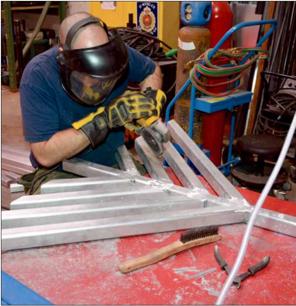
MCpl Chris Lagace grinds welds on the menorah being constructed at 17 Wing for lighting during Chanukah. Please see the story on page 15 for more information about the lighting. Photo: Cpl Adam Blundon, WCE.
