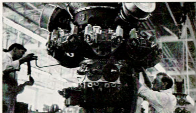
Final assembly of a commercial airliner's turbo compound engine takes place at Bristol's Montreal Plant.
