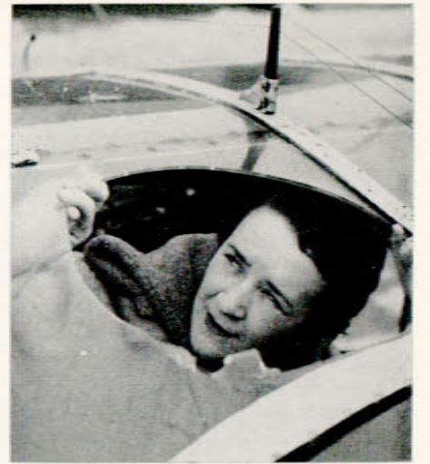
PANICKY DUCK smashed this 14-inch hole in an Air Ambulance windshield on a flight to Estevan. Air ambulance survived, duck didn't. —Sask. Gov't Photo.
