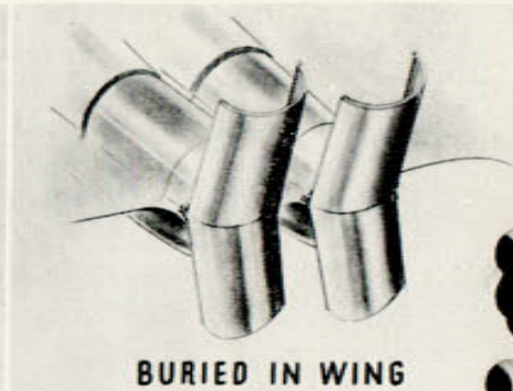
Possible reverser installations for three types of jet engine installations are shown in the drawings above. The "Clamshell W" jet thrust reverser illustrated were the most promising type studied by Boeing engineers in a three-year search for a means of using jet thrust to decelerate airplanes after landing.
