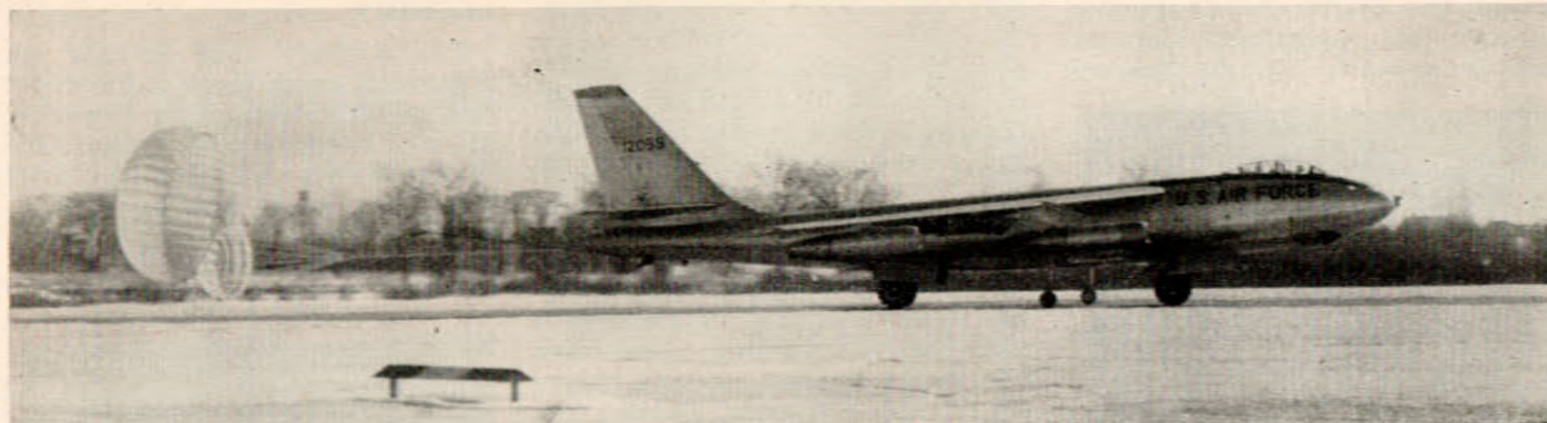
It's two parachutes braking it, the first B-47 Boeing Stratojet ever to land at Montreal comes to a stop on Cartierville airport, Montreal, to enter the plant of Canadair Limited, where it is being fitted, on a unique design, with a seventh jet engine—a newly-developed Orenda. The plane, on a two-year loan from the United States Air Force to the RCAF, will be used as a flying test-bed for the seventh engine. At the end of its 1,400-mile 150-minute flight from Wichita, Kansas, the B-47 came to a stop in less than half the length of the 6,350-foot Cartierville runway.
