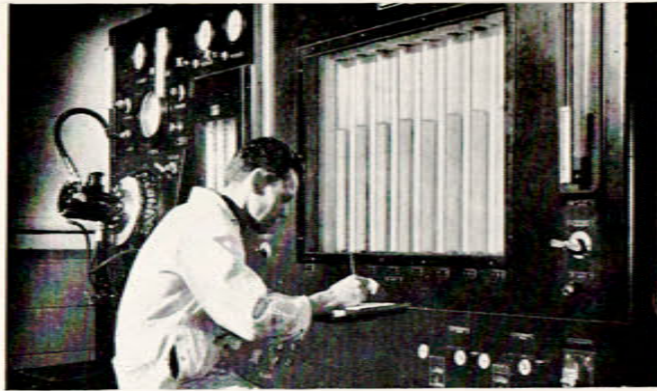
This modern test equipment calibrates the overhauled fuel system prior to final assembly.
