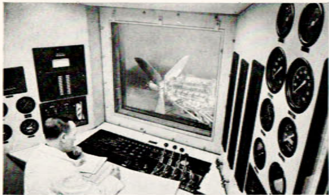
All details of engine behaviour and performance are checked in these well-equipped test cells, which are also the largest of their kind in Canada.
