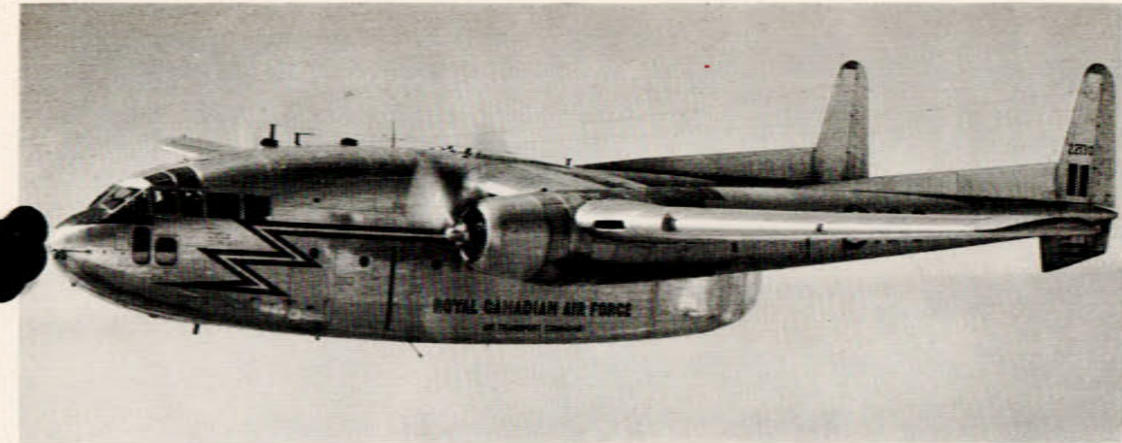
"Fairchild C119 "Flying Boxcar" powered by two Wright R3350-85 Compound Engines.
