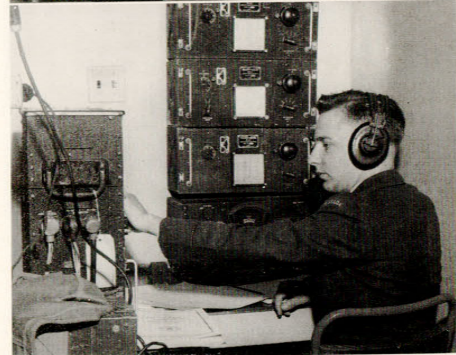
F/C G. L. McPhee, student of the Long Range School, uses the APS 33 airborne radar on a training flight.
