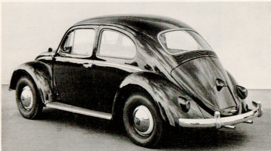
A little change, notably by the increased glass area in the rear, and a better heater for North American use. Minor changes in the interior.
