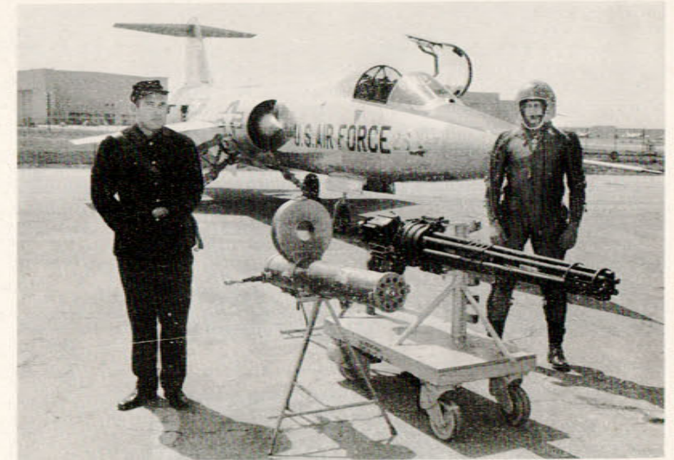
SOMETHING OLD, SOMETHING NEW—Something borrowed and something capable of blasting hostile aircraft right out of the blue. This "then-and-now" photo depicts one of the most remarkable development cycles in military history—a Civil War weapon (designed 95 years ago) adapted to arm the fastest jet fighter in the sky, Lockheed's F-104A Starfighter. Called the Gatling Gun, after its inventor, the tripod-mounted weapon was manually "cranked" by an infantryman attired like the model at left. Today's jet pilots flying the ultra-sonic Starfighter (background) have at their fingertips armament including the most potent aerial cannon ever developed—the rapid-firing, six-barreled 20-mm. Vulcan—a 20th century version of the weapon which revolutionized military firepower nearly 100 years ago. Both guns feature a rotating cluster of barrels and both are externally powered. In contrast to its predecessor's manual operation, the Vulcan is powered electrically. Being built by General Electric, the Vulcan can unleash 10 times the firepower of World War II fighter machine guns.
