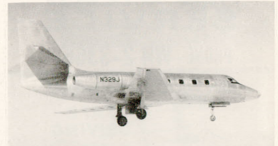
GEAR DOWN AND LOCKED—First aerial view of Lockheed's new JetStar, in landing pattern at Edwards Air Force Base, emphasizes 34-degree sweep on the leading edge of its 53-foot wing. Main landing gear of JetStar—America's first jet utility transport—retracts into mid-fuselage wheel wells; nose gear retracts forward. Photo also clearly shows wide clearance of jet exhausts under high-mounted horizontal stabilizer. The JetStar flies at 500 to 550 miles an hour. The first prototype, powered by two Bristol Orpheus engines mounted in pods at each side of the rear fuselage, is undergoing instrumental aerial tests at Edwards. A second prototype will use four General Electric J-85 or Fairchild J-83 engines. The 10-passenger jet made its first flight September 4—just 241 days after go-ahead development signal was given. Designed as an off-the-shelf item specifically to meet Air Force trainer-transport requirements, the JetStar has a two-man crew, normal cruise range of 1,700 miles at 40,000-foot altitudes, and is completely air-conditioned and pressurized.
