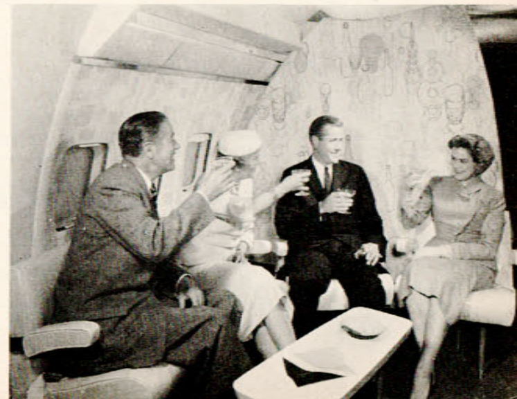
The aft lounge of the Boeing 707-120 Stratoliner interior mockup. Adding to the versatility of the transport interior is the partition in the background which fits into the slots in the floor which also hold the seats. Conditioned air enters the cabin through the perforated light fixture cover above the windows. Air circulates through the cabin and is withdrawn through slots at floor level. The half-million-dollar mockup was prepared to provide airlines that have ordered Boeing 707 Stratoliners and Intercontinentals a means of visualizing the potentialities of the transports' interiors.
